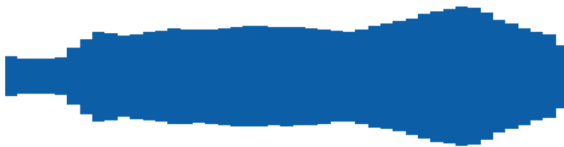
Figure 2: A 44 section vocal tract representation using the resting diameters given in Appendix A of Story, 2005 [4]. Each section acts as a resonator perturbing the glottal wave.
